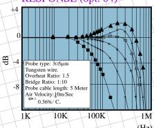
The typical frequency response graph was plotted according to data taken from AN-1003 Hot-Wire Anemometer with options 01 & 04. The amplitude is relative to the amplitude @ 1 KHz.
